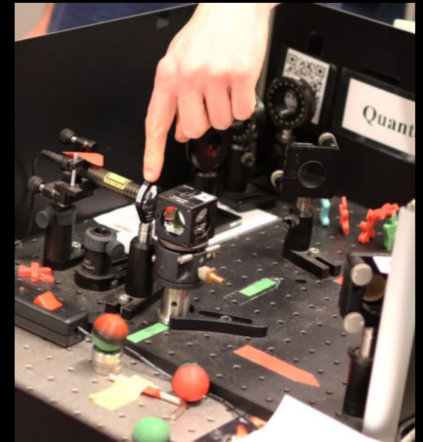
3. Mach-Zehnder-Interferometer as I-Qubit-Quantumcomputer
